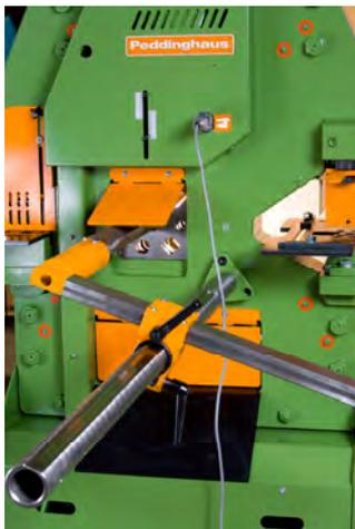
Universal electrical contact length stop, for 1 metre cutting length
