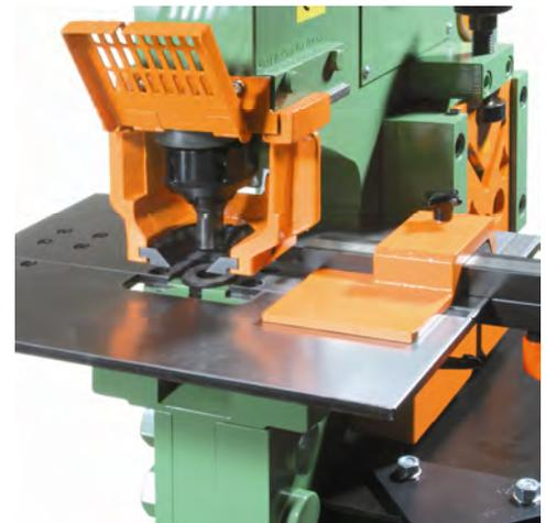
Material support table, 500 x 405 mm, with mm graduation, slot-in front section, to suit the standard punching attachment
