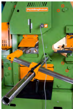
522 electrical contact length stop 1, 2 or 3 metres
