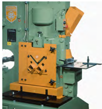
549 hydraulic hold-down for the section shear and flat shear
