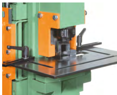
703 for the notcher side: special attachment for punch no. 7, die no. 6, equipped with corner radiusing tool, R = 35 mm
