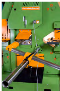
522 electrical contact length stop 1 meter 2 meters 3 meters
