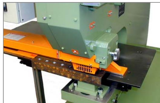
Gauging table, front part removed, for punching angle iron
