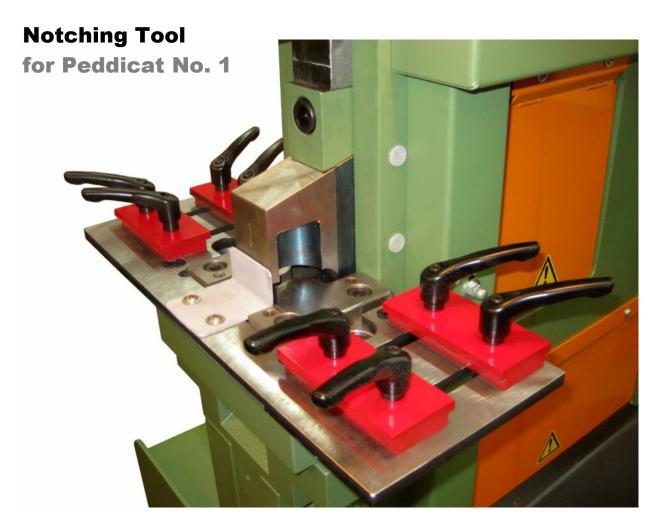
Shearing and double-sided radiusing tool
